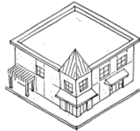
Side and rear elevations should not be blank (top). Instead, façade ornamentation should wrap corners (middle).
